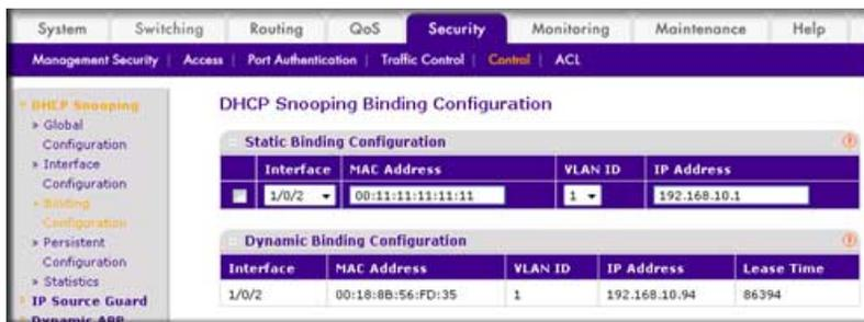
2. Fill in the fields for the static binding and click **Apply**.
