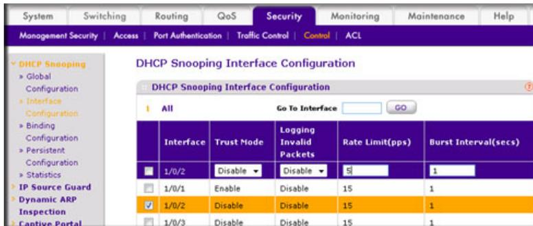
2. Select the interface, fill in the **Rate Limit (pps)** field, and then click **Apply**.
