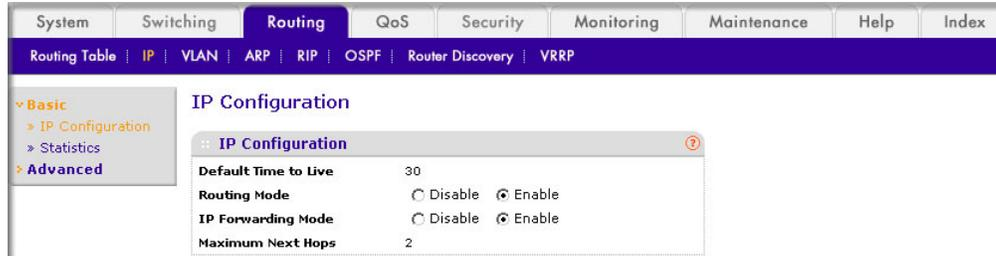
2. For Routing Mode, select the **Enable** radio button.
