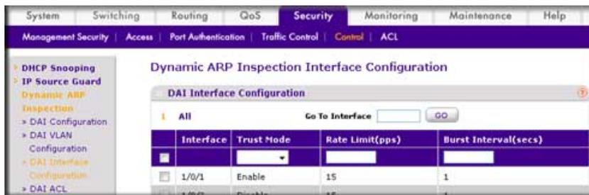
Now ARP packets from the DHCP client will go through; however ARP packets from the static client are dropped, since it does not have a DHCP snooping entry. It can be overcome by static configuration as described in the following section, [Static Mapping](#) on page 303.
