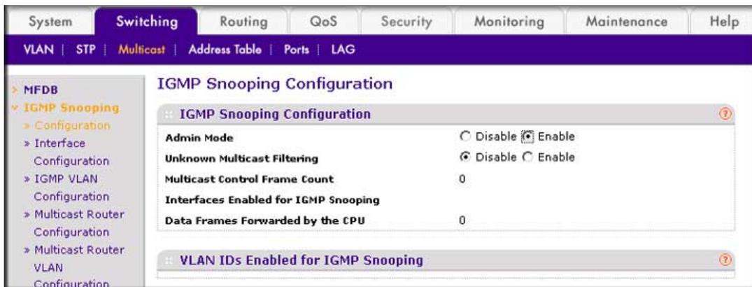
2. Enable IGMP snooping on VLAN 1.
