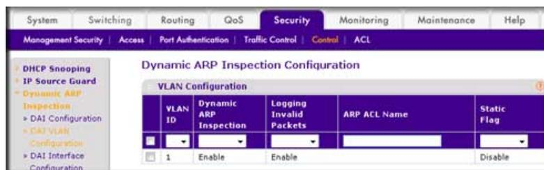
Now all the ARP packets received on the ports that are member of the VLAN are copied to the CPU for ARP inspection. If there are trusted ports, you can configure them as trusted in the next step. ARP packets received on the trusted ports are not copied to the CPU.
