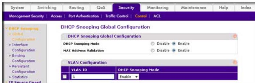
3. Configure the port through which the DHCP server is reached as trusted.
