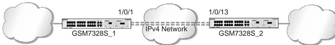
Figure 44. 6in4 tunnel between two switches
