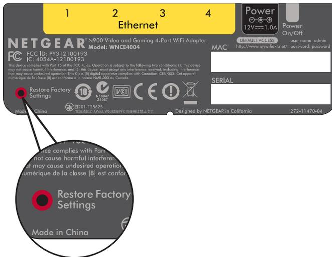
Figure 3. The Reset button restores factory settings
