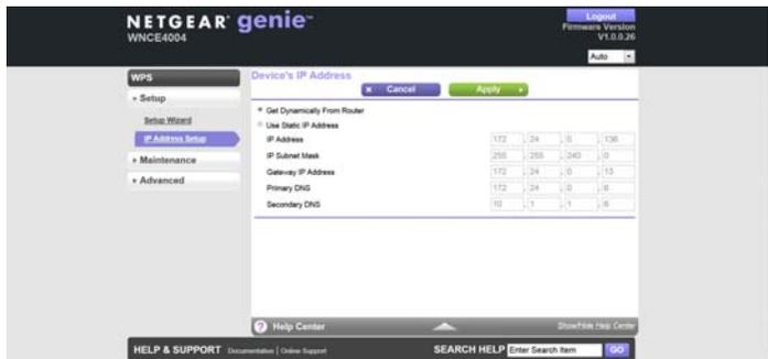
This screen shows whether the Internet adapter is set to get its IP address dynamically from the router (this is the most common setting), or is set as a static IP address.
