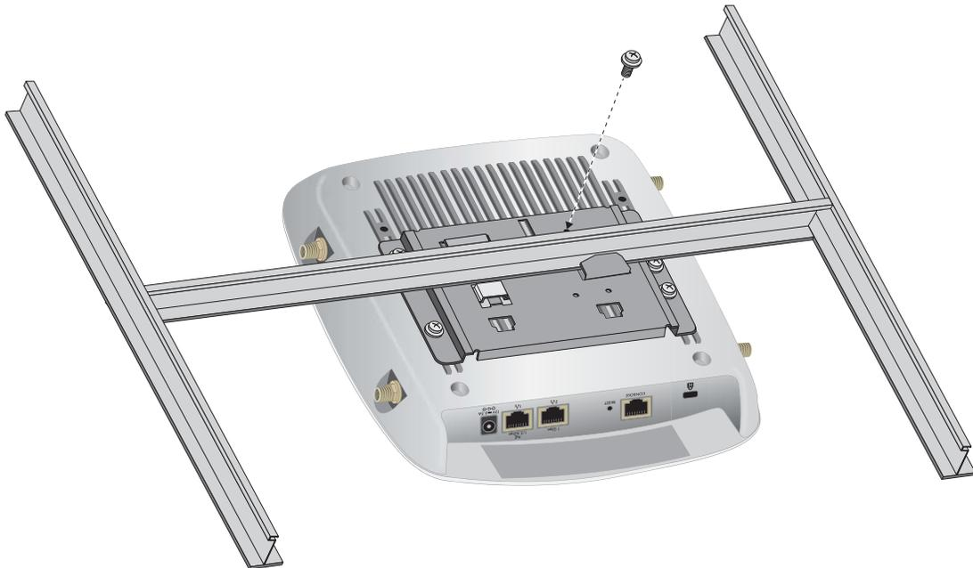
4. Secure the access point to the ceiling rail using the T-bar screw.
