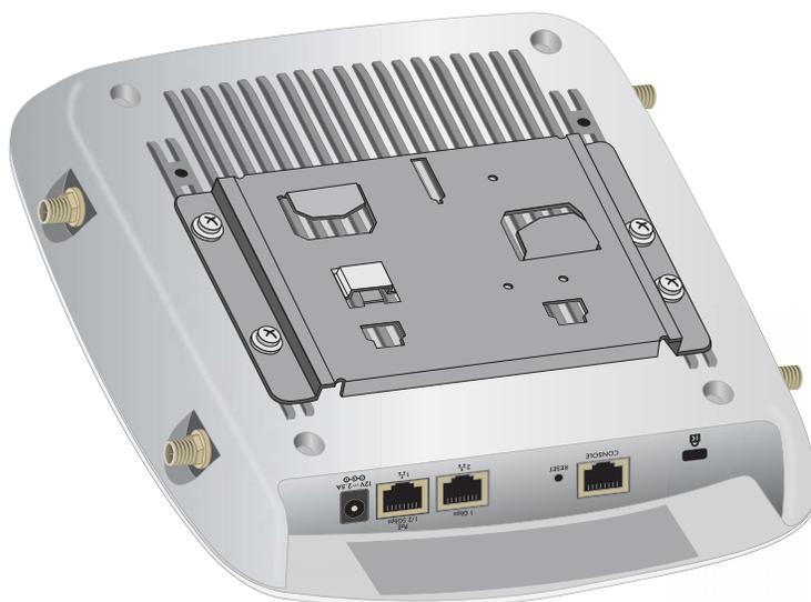
4. So that you can see how the brackets fit together, attach the wall-mounting bracket to the access point–mounting bracket as shown in the following figure.
