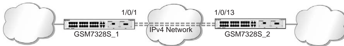
Figure 44. 6in4 tunnel between two switches
