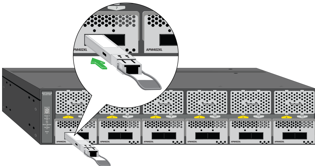
Figure 8. Inserting a QSFP transceiver module
