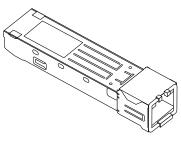
The AXM765 SFP+ module is a low-power, high-performance, multigigabit 10G/1000BASE-T/100BASE-TX transceiver. The AXM765 delivers 10 GbE network connectivity with cabling up to 98.5 feet (30 meters) and delivers 1G/100M network connectivity speed through 92.8 feet (100 meters) of Category 5e (Cat 5e) or Cat 6 Ethernet cable.
