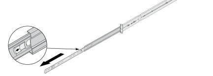
The inner rail slides out and separates from the middle rail.
