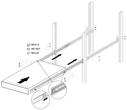
The inner rails continue sliding into the middle rails.
