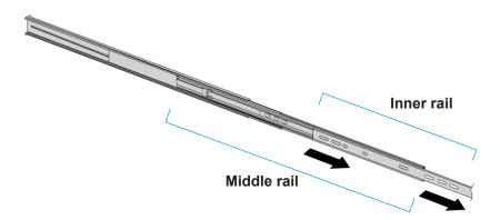
2. Press the release latch on the middle rail and adjust the middle rail so that the three holes at the front of the outer rail are visible.
